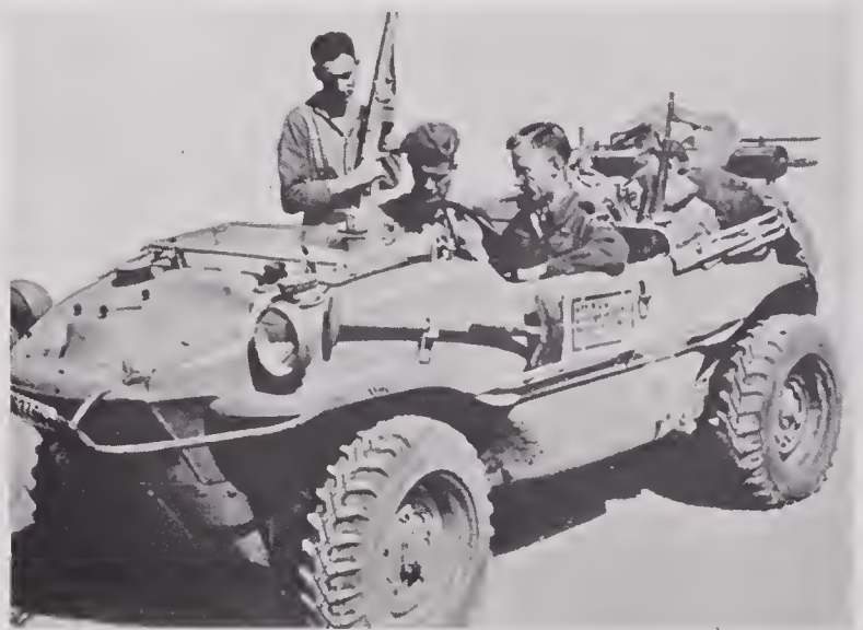
FIGURE 17. German amphibious wheeled scout car, captured in France in 1941, propelled by retractable outboard drive. Marine power provided by mechanical power take-off from vehicle engine.
